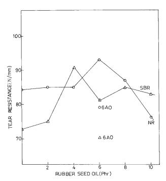
Figure 7 Variation of tear resistance with oil content.
