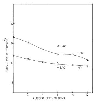
**Figure 4** Variation of crosslink density with rubber seed oil content.
