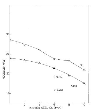
Figure 5 Variation of modulus with oil content.
